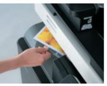
Optional Job Separator trays separate print/fax output from copy output.
